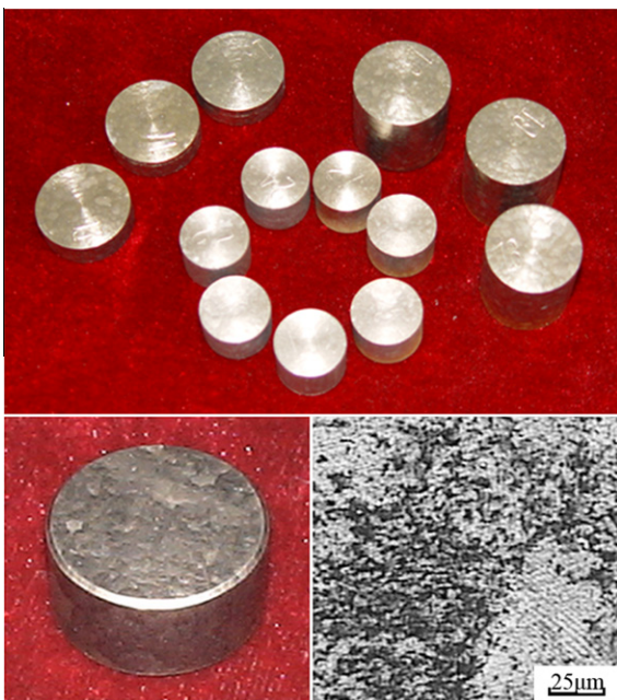
Fig. 9. Images and micrograph on surface of the crack-free zirconium hydride samples.
